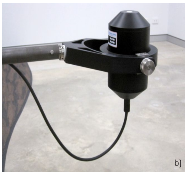
Figure 1. (a) The DALEC instrument is mounted at the end of the boom extending from the foremast of the Southern Surveyor over the bow of the vessel (b) Close-up of the DALEC sensor head
