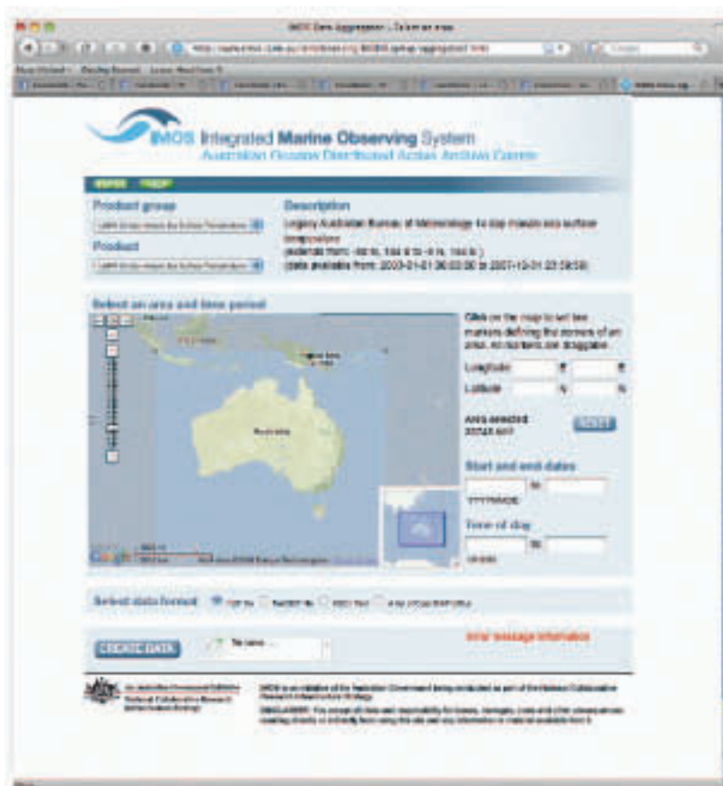
Figure 4. The web interface to the prototype AO-DAAC aggregator service enables selection of data sets, as well as geographical and temporal bounds. All data matching the request specification is retrieved and written to an output file in HDF, netCDF or ASCII format that is then provided to the user.
