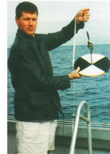
Curtin University student Andrew Rodger with a Secchi Disc for measuring the turbidity of Perth waters.
