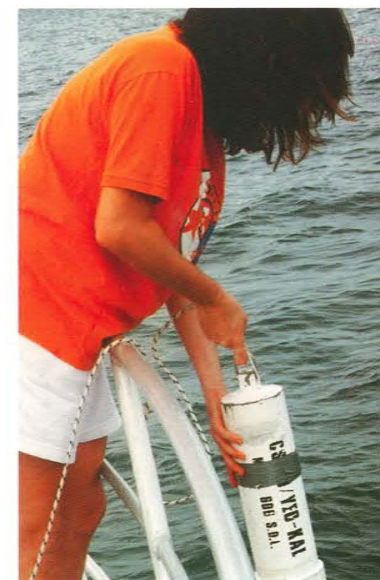
CSIRO oceanographic assistant Angela Way lowering an electronic probe into the water to measure temperature and salinity profiles of the ocean off Perth
