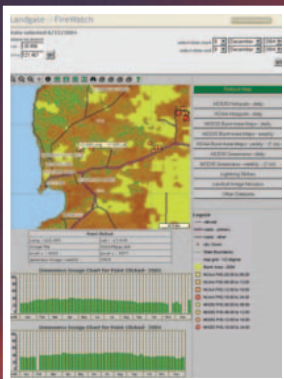
Figure 2: Example from the FireWatch website firewatch.dli.wa.gov.au, showing the fire hotspots (shown in red symbols), burnt area (green) and NDVI time series. The image backdrop is the NDVI from the corresponding MODIS overpass. The graphs allow the user to compare the change of NDVI across and between seasons.
